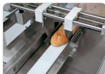
Intermittent belted infeed conveyor
